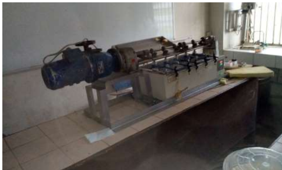
FIGURE 1: A locally-fabricated fermentor used for the liquefaction.
